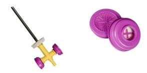
The G/O Safety filter vent assembly is used to filter displaced air exiting a collection vessel as it fills with contaminated liquid. It may be used during the transfer of liquids for temporary storage or permanent disposal.
